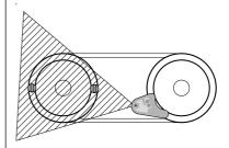
Targets placed for Horizontal alignment.
